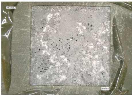
Fig.5 Results of pitting corrosion observation.
