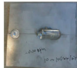
Fig.2 FSW joined aluminum plates. (A5052)
