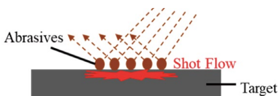
Fig.18 Schematic image of blast surface treatment.
