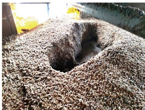
Fig. 7 The photo of hole in filler layer at demonstration test.
