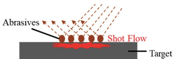
Fig.18 Schematic image of blast surface treatment.
