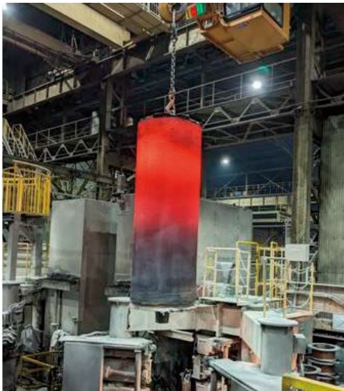
Fig.13 Photo showing typical manufacturing scene of upper pinch roll by CPC.
