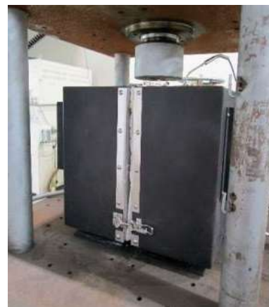
Fig. 3 Photograph showing furnace for mold heating.
