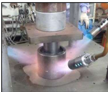
Fig. 2 Photograph showing mold being heated by gas flame.
