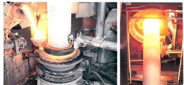
Fig.4 CPC process in operation, (a) Overview of pouring, (b) Appearance of just as-cast product.
