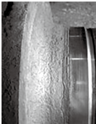
Fig.2 Appearance of the corroded journal
