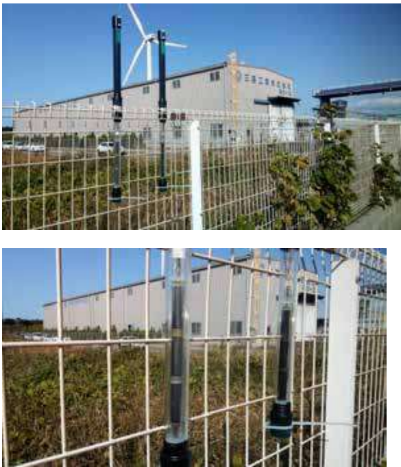
Fig.12 Wireless sensor with cylindrical PV system operation test in outdoor environment.
