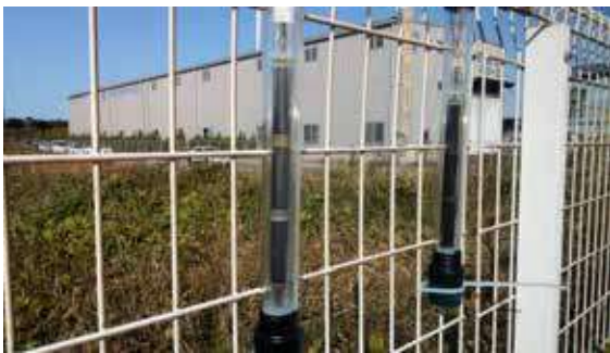
Fig.12 Wireless sensor with cylindrical PV system operation test in outdoor environment.
