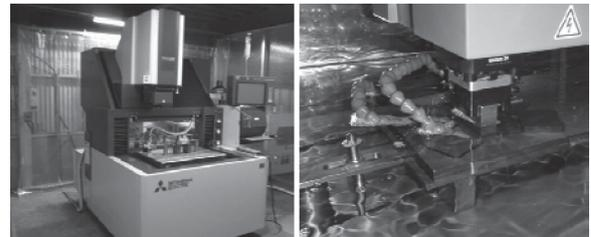
Fig.6 3-axis CNC electric discharge machining center
