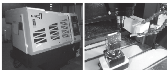
Fig.7 3-axis CNC high-precision machining center
