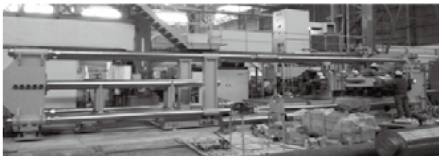
Fig.1 Photo showing developed friction welding device
