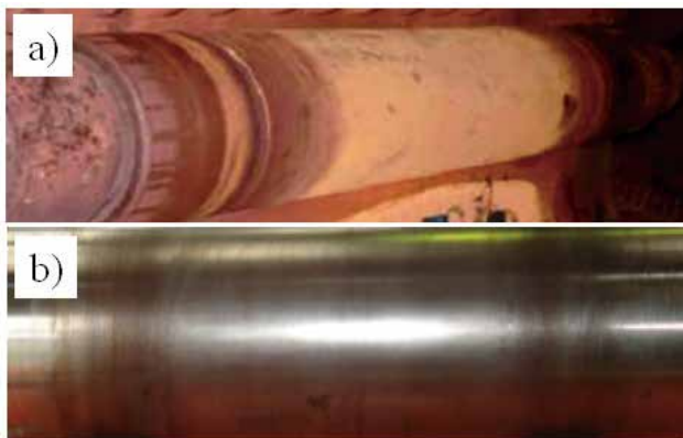
Fig.9 Wrapper roll appearance: a) conventional alloy, b) FKS-KC5 6)
