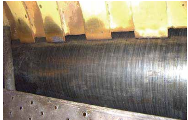
Fig.2 Bead-mark observed in wrapper roll
