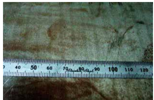
Fig.3 Print of bead-mark to strip
