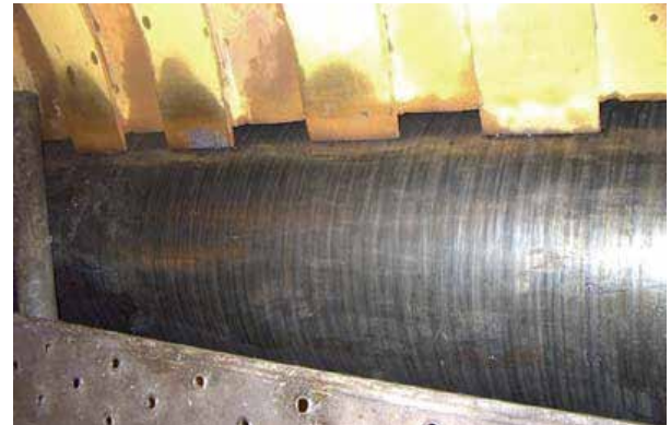
Fig.2 Bead-mark observed in wrapper roll
