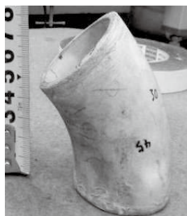
Fig.16 Elbow pipe of Al 2 O 3
