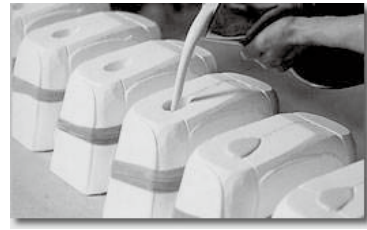
Fig.17 manufacturing process of Al 2 O 3 pipe by casting method
