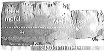
(b) Melting loss of base metal
