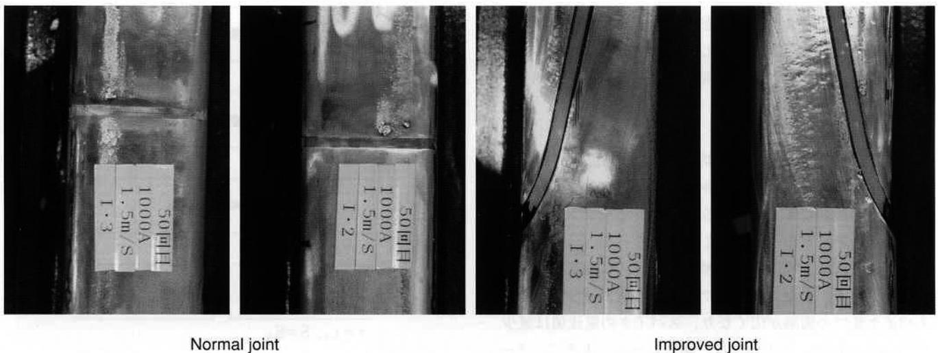
Fig.5 Arc-mark around the rails joint
