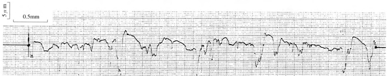
Fig.3 Roughness of roll surface after rolling (F3, 5069 ton) (Ra = 2.9 \mu m, Rmax = 24.6 \mu m)
