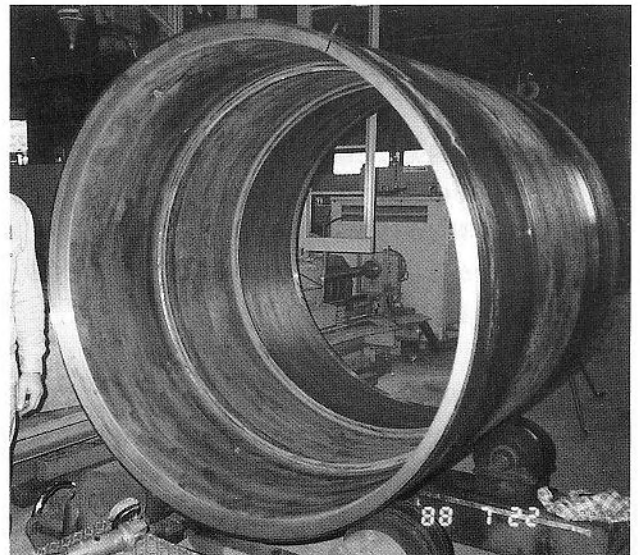
Fig. 10 View of shell after sand removing
