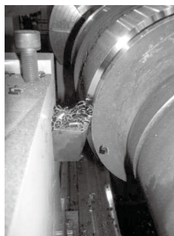
(b) Machining for regeneration work roll
